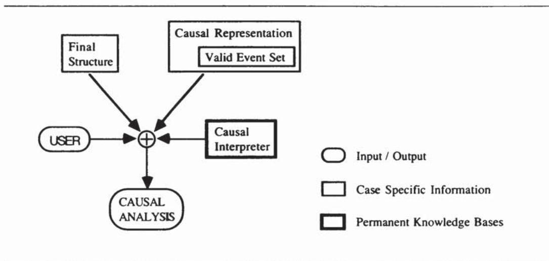
The Causal Interpreter provides a procedural means of eliciting the required analysis from the Causal Representation and Final Structure. In this case the goal is primarily to produce Cause and Symptom Equations (CSEs).
