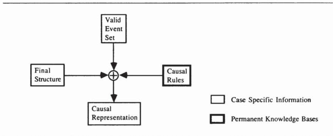
Here the final structure representation of the process is available, and a complete set of the events which will appear in the causal analysis has been constructed. The next step is to develop causal links between these events; this is done by the application of causal rules. The representation system used for describing causality in the KBS and the application of causal rules to determine fault propagation characteristics are discussed in the next two sections.
