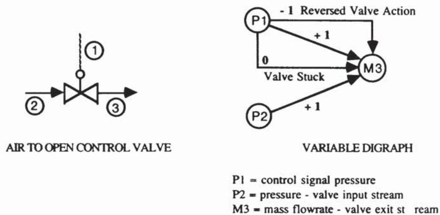
The complexity of the digraphs representing a component depends, naturally, on the number of variables and failure modes considered.
