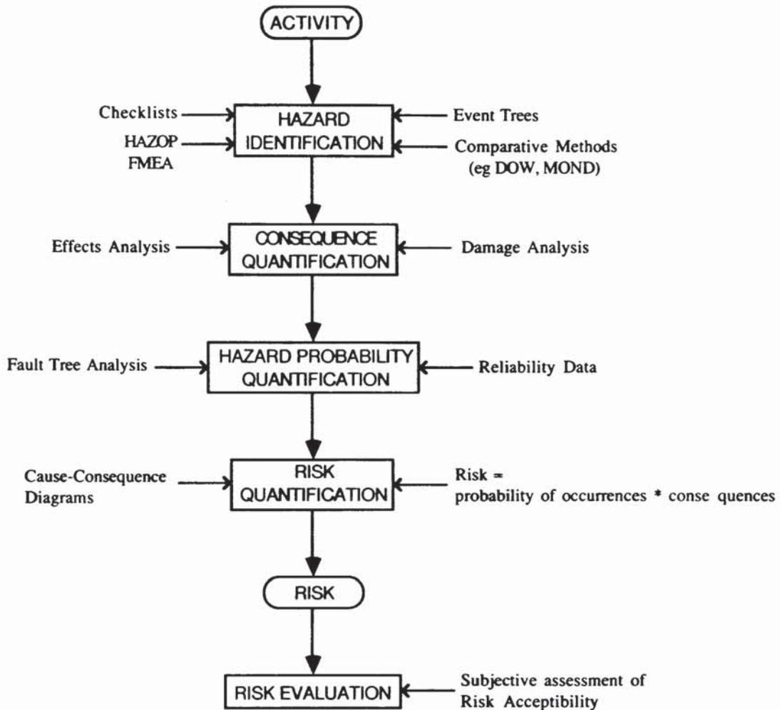
As may be seen from Figure 2.3.2a, Risk Assessment involves a number of techniques which analyse the propagation of faults in process plant: HAZOP, Event Tree Analysis, FMEA and Fault Tree Analysis.
