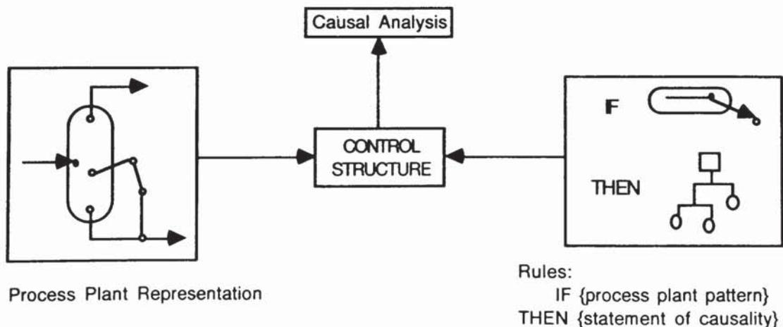
Any rule based system for causal analysis must have the overall characteristics shown in Figure 5.1a:
