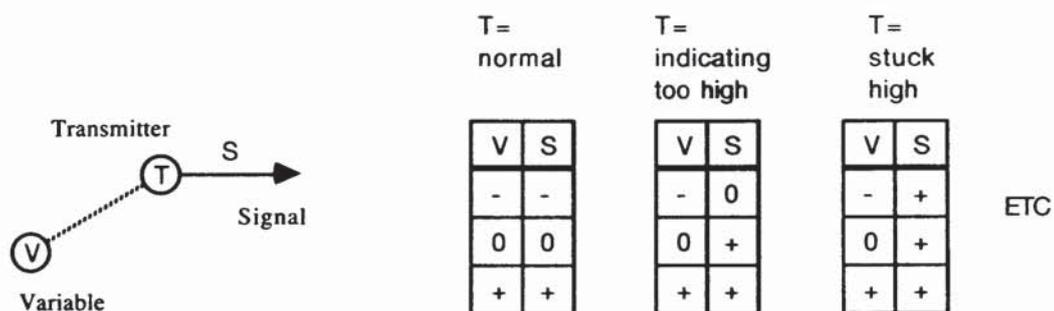
This representation of a device as an object with a clearly defined set of inputs and outputs suggests that a symbolic simulation of an object may be created; given input variables and the object state, the simulation would produce the outputs. This could be implemented using Object Orientated Programming, as discussed in Section 3.5.2.
