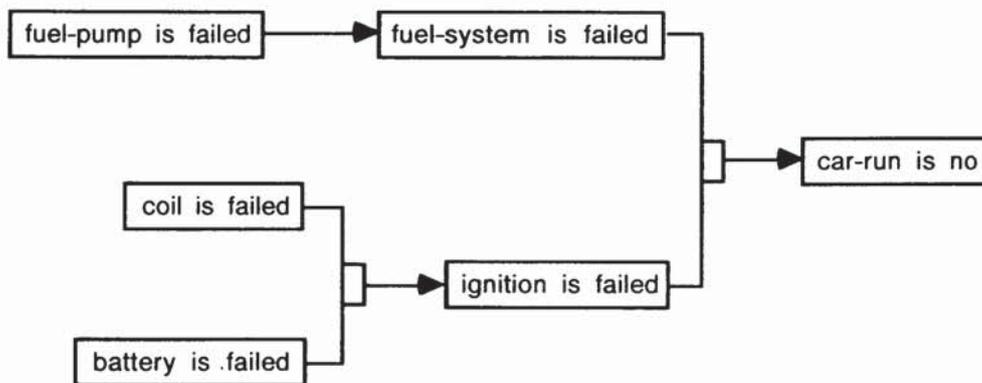
This tree representation of the relationships between concepts may be constructed first, and the equivalent rules derived from it.
