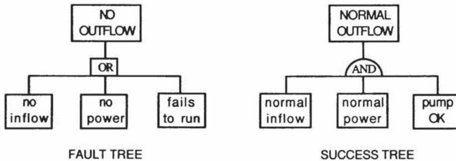
The coupling of components is achieved by defining a set of 'nodes' throughout the system. The output from each component is connected to a node which is, in turn, connected to the inputs of one or more succeeding components; this provides for divergence in fault propagation. Thus an output event of a component can be said to occur at its output node; this nodal event corresponding with input events of succeeding components.
