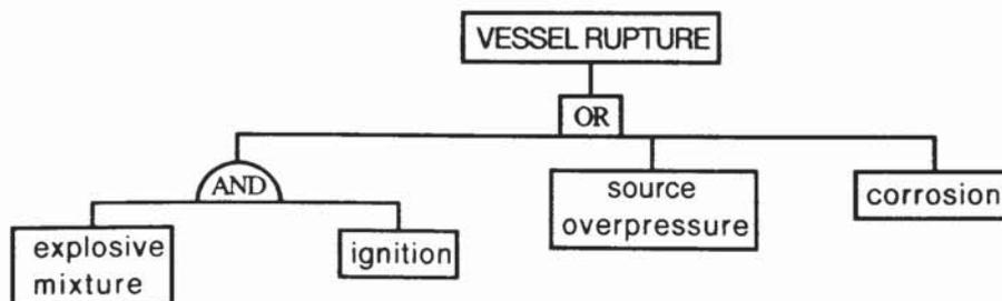
FIGURE 2.5.2a A Simple Fault Tree
