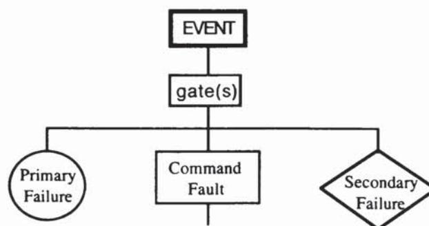
Applying this "gate template" in conjunction with the component failure characteristic diagram Figure 2.5.3b [Henley 1981] assists in developing the causes of a particular event.
