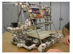
Figure 5: RepRap v.2 'Mendel' fused deposition modelling 3D printer (Credit: Wikipedia /Charles C)
