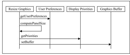
Figure 2. A simple sequence diagram, "Resize Graphics."
