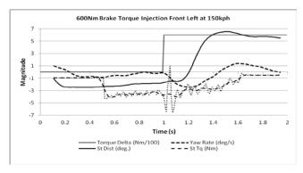
Figure 2: EV1 dynamic response to torque fault injections
