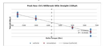
Figure 5: yaw rate data for EV1, vehicle observations compared with simulated results.
