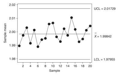
Fig. 18-2 X-bar chart for width.
