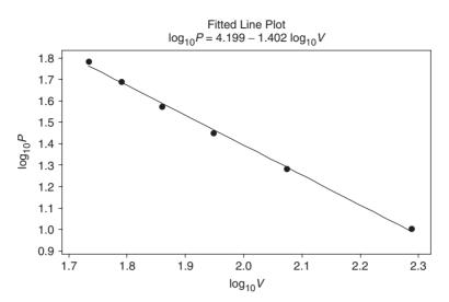
Fig. 13-15 Reducing nonlinear equations to linear form.
