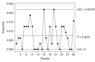
Fig. 18-5 The *P*-chart monitors the percent defective.
