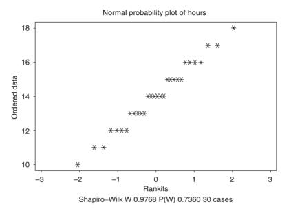
The normal probability plot is shown above. The Shapiro–Wilk statistic along with the *p*-value is shown. P(W) = 0.7360. Since the *p*-value is considerably larger than 0.05, normality of the data is not rejected.
