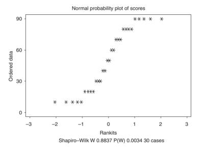
The normal probability plot is shown above. The Shapiro–Wilk statistic along with the *p*-value is shown. P(W) = 0.0034. Since the *p*-value is less than 0.05, normality of the data is rejected.
