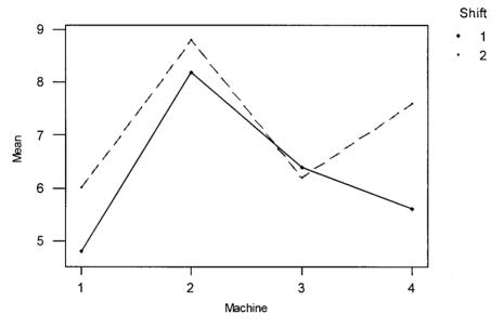
Fig. 16-7 Interaction plot—data means for defects.
