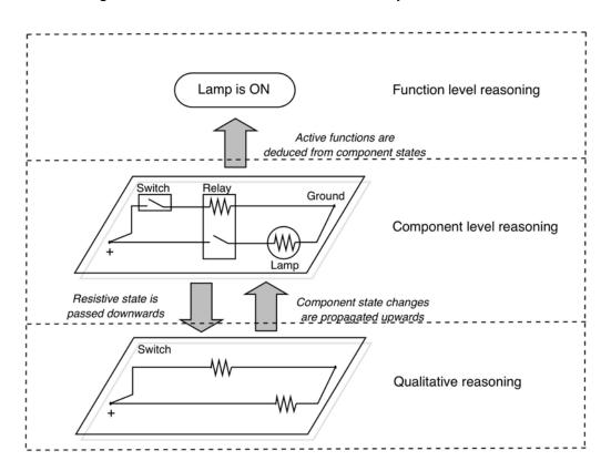
Fig. 1. Levels of electrical simulation
