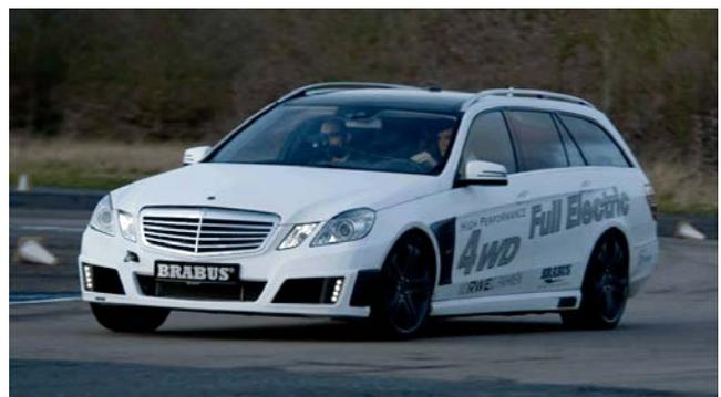
Figure 1: Brabus 4WD vehicle (EV1) fitted with Protean Motors during fault injection testing (Photo D. Harty).
