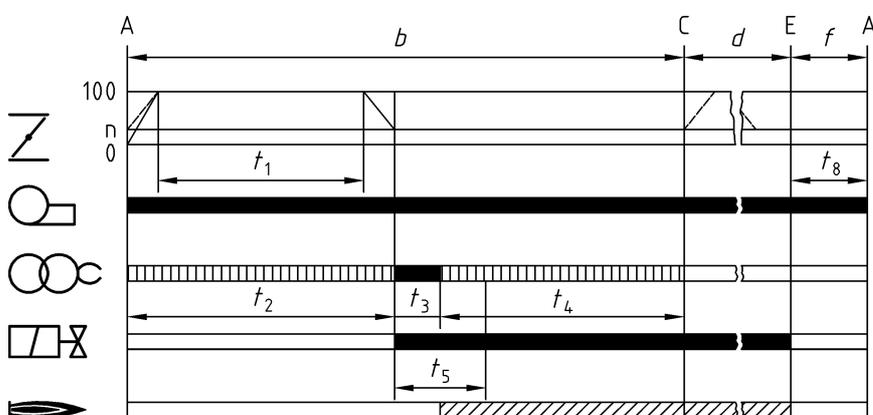
c) Supervised air damper operation, operation with post-purge
