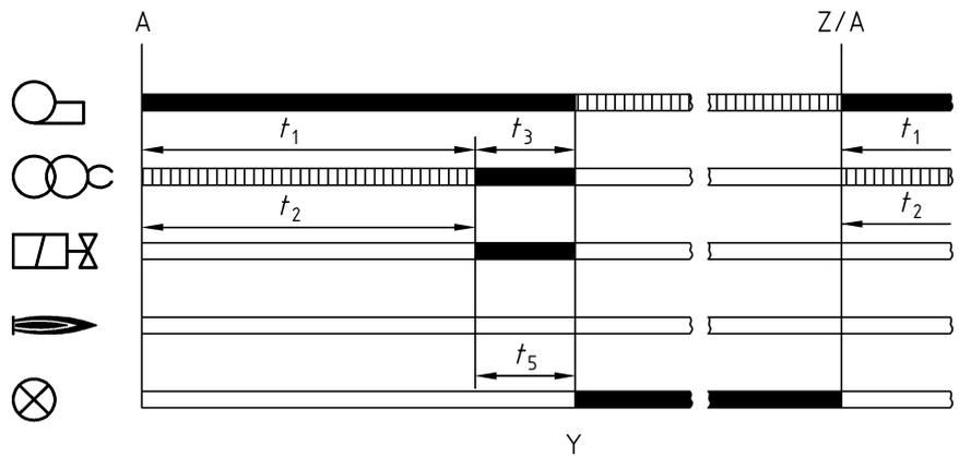
Figure D.6 — Lock-out for the non-establishment of the flame signal (during safety time  $t_5$ )
