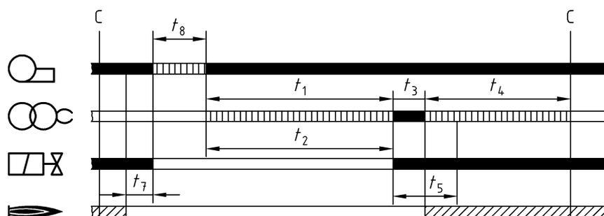
Figure D.4 — Re-cycling after extinction of flame during operation
