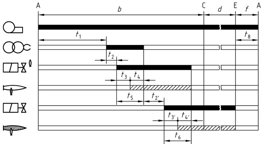
a) Pilot **supervised**, operation with post-purge two main valves in series or see EN 267
