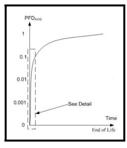
Figure 2 PFD<sub>AVG</sub> and Valve Life Cycle
