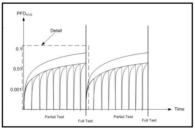
Figure 3 PFD<sub>AVG</sub> is decreased due to PST combined with full cycle testing
