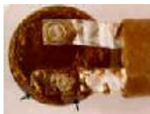
Inside a failed electrolytic capacitor showing a broken positive connection at the right arrow and contamination around the rivet at the left arrow
