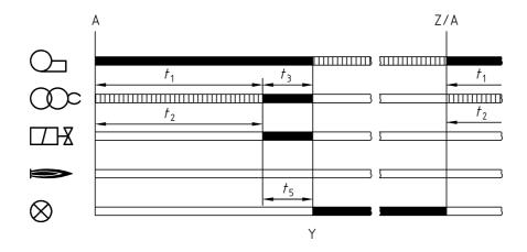
Figure D.6 — Lock-out for the non-establishment of the flame signal (during safety time  $t_{\rm 5}$ )
