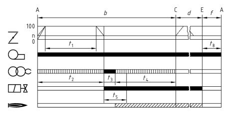
c) Supervised air damper operation, operation with post-purge
