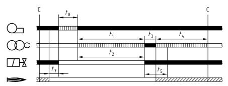
Figure D.4 — Re-cycling after extinction of flame during operation
