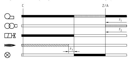
Figure D.5 — Lock-out after extinction of flame during operation
