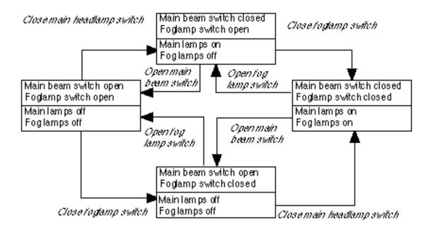
Figure 5.3: State graph for simple car lighting circuit
