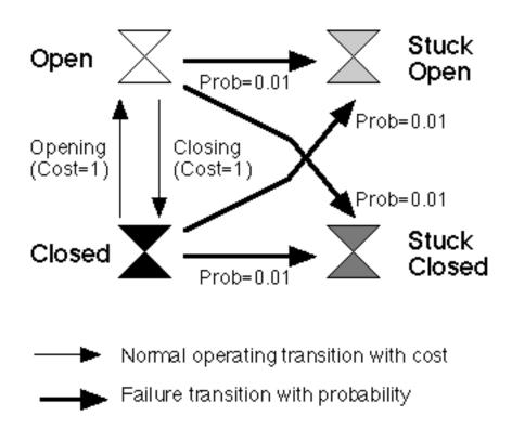
Figure 6.11: Component model for a valve (Taken from [Williams and Nayak])
