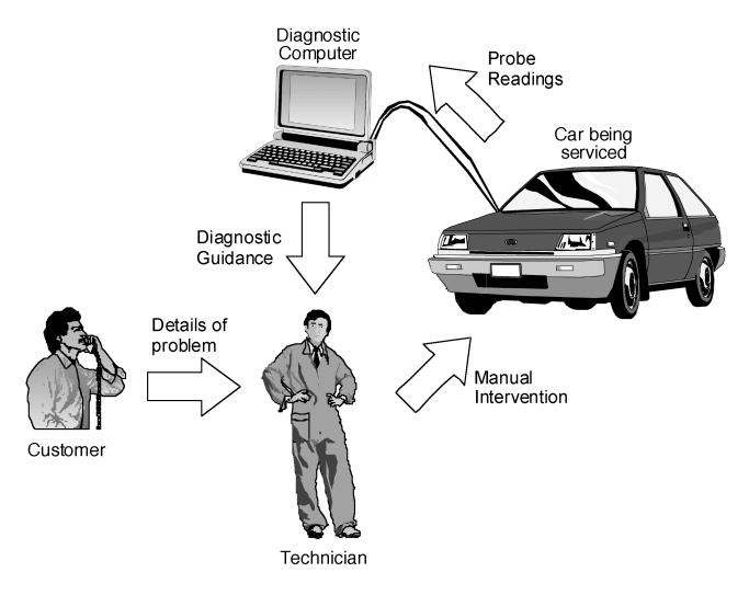
Figure 3.6: Use of garage-based diagnostic system
