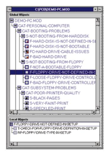
Figure 3.2: Display of fault tree in TestBuilder
