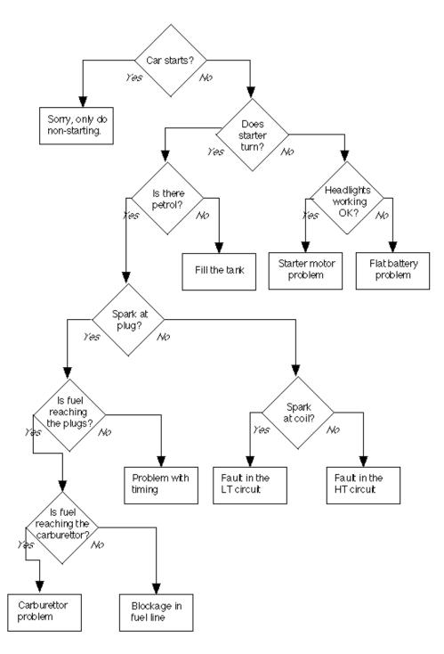
Figure 1.1: A simple diagnostic fault tree
