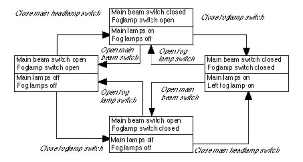
Figure 5.4: State graph for faulty car lighting circuit
