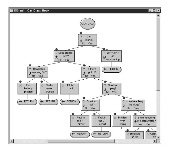
Figure 3.7: Simple car diagnosis system in GRADE
