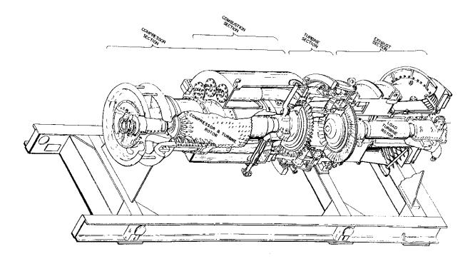
Figure 7.1: Main components of a gas turbine
