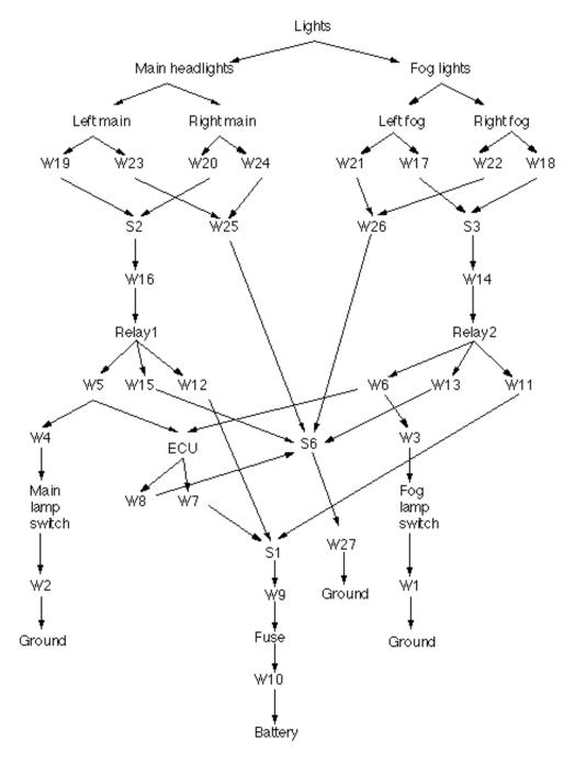
Figure 5.2: Dependency graph for simple car lighting circuit
