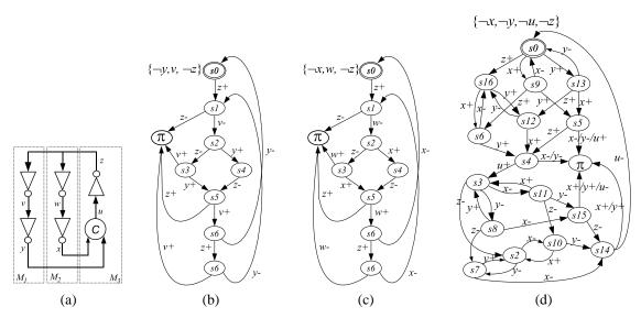
Fig. 3. (a) Block digram of a simple asynchronous circuit. (b) - (d) The SGs for module  $M_1$ ,  $M_2$ , and  $M_3$  where the inputs of the components are set to be completely free.
