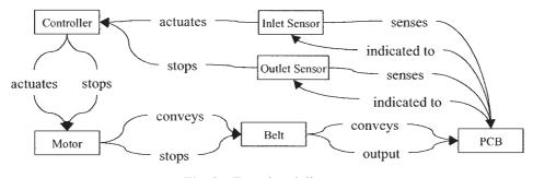
Fig. 8 Functional diagram
