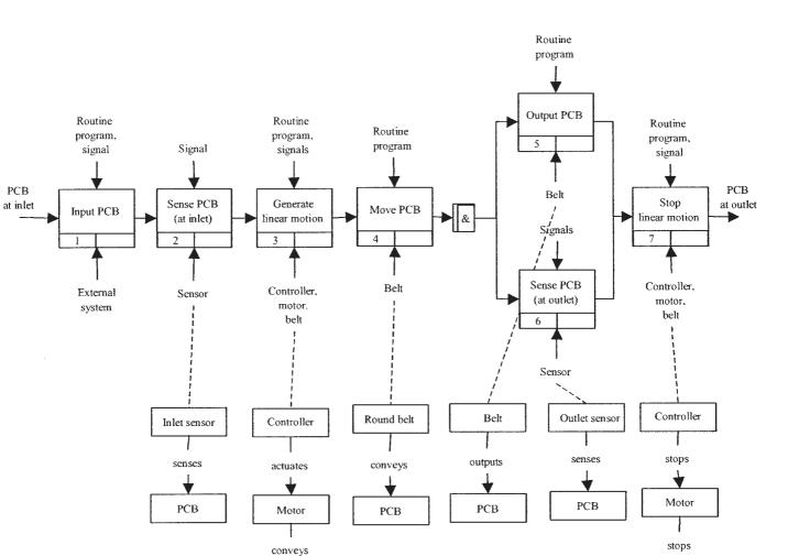
Fig. 7 Function and structure mapping
