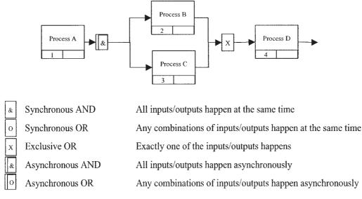
Fig. 4 IDEF3 diagram with logical connectors
