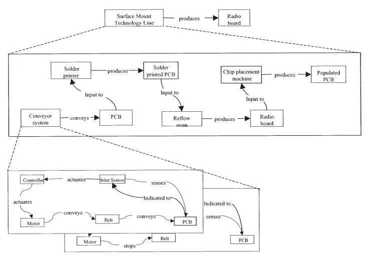
Fig. 10 FMAG model decomposition
