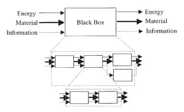
Fig. 2 Functional model with energy, material and information flows
