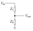
Figure 4: Voltage Divider
