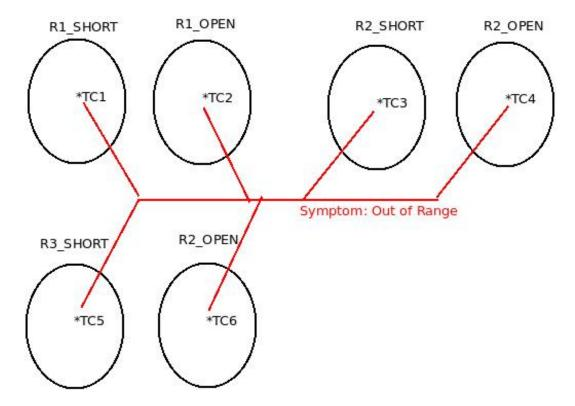
Figure 5: PT100 Component Failure Modes
