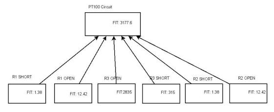
Figure 7: Probablistic Fault Tree : PT100 Single Faults
