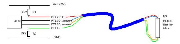
Figure 1: PT100 four wire circuit
