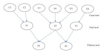
Figure 5. "Signal Interference" FMEA converting to BN2
