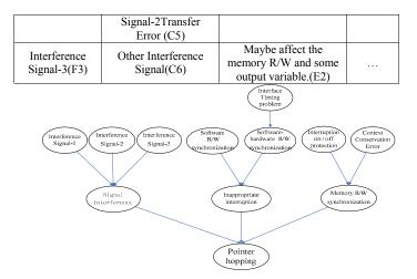
Figure 4. "Pointer Hopping"FT converting to BN1
